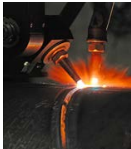
Pre-heating during cutting
