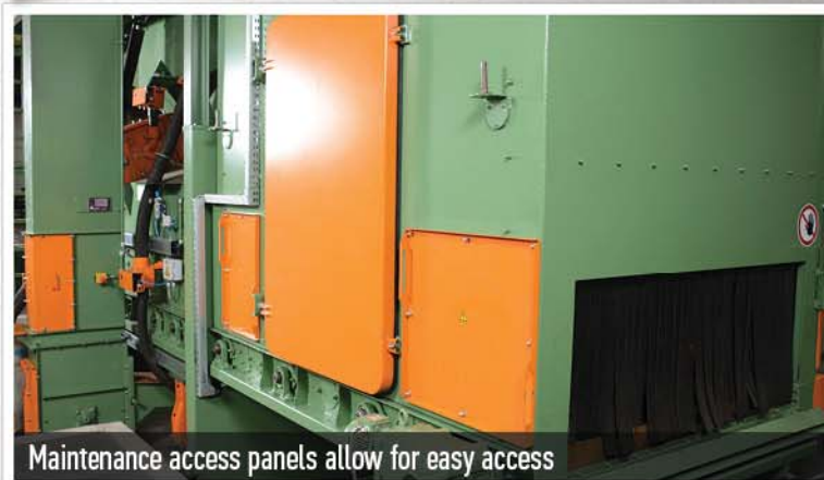
Abrasive containment curtains keep shot inside machine
