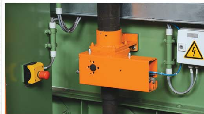
Shell valves reduce wear on turbines and blast chamber
