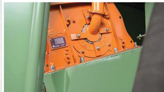
Turbines built from tough manganese and tool grade steel
