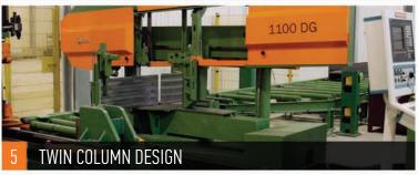
Rugged twin column construction eliminates vibration and is critical for cut quality and blade life
