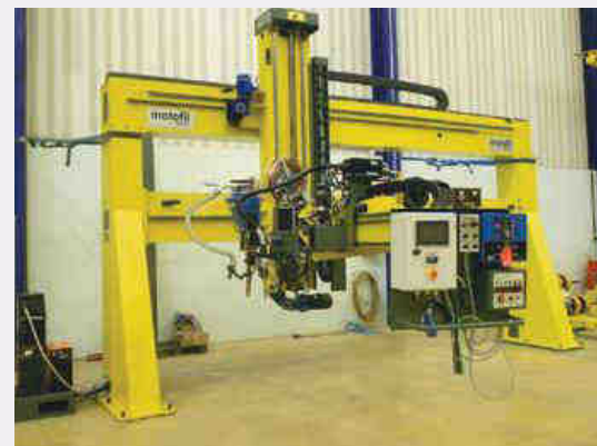
AUTOMATED WELDING GANTRY
