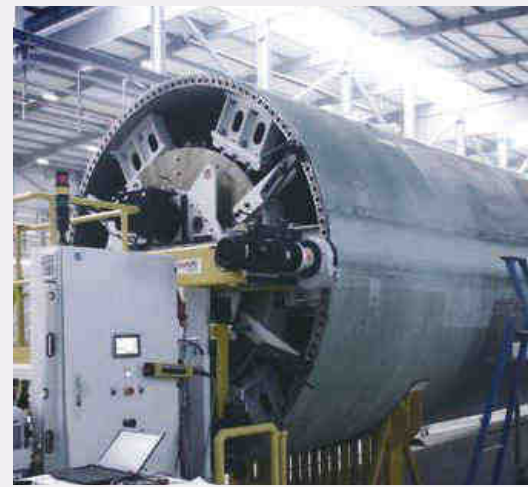
BLADE GRINDING MACHINE FOR WIND TURBINE TOWERS
